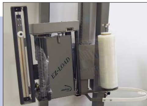
Standard Machine Carriage with Optional Pneumatic Roping Device
