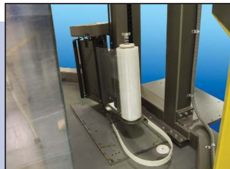
EZ-LOAD Carriage Assembly with Safety Hoop
