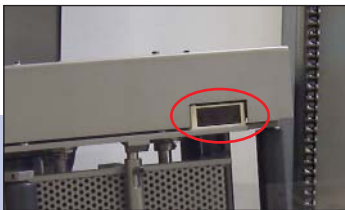
Guarded Photo Electronic Load Height Sensor
